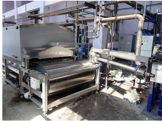
The Esiform is fixed to the belt frame using a pivoting point and can be hinged away from the belt to the cleaning position for cleaning, maintenance or changing the perforated tube.
